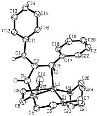
**Figure 3.** ORTEP diagram of compound **8.** Most hydrogen atoms have been removed for clarity; selected bond distances, Å and angles °: C1–C2 1.382(2), C2–C3 1.416(2), Li–C3 2.370(3), C1–C2–C3 130.92(12), C4–C2–C3–Li 54.92(12), C2–C3–C17–C18–15.3(2), C2–C1–C11–C16–14.8(2).
